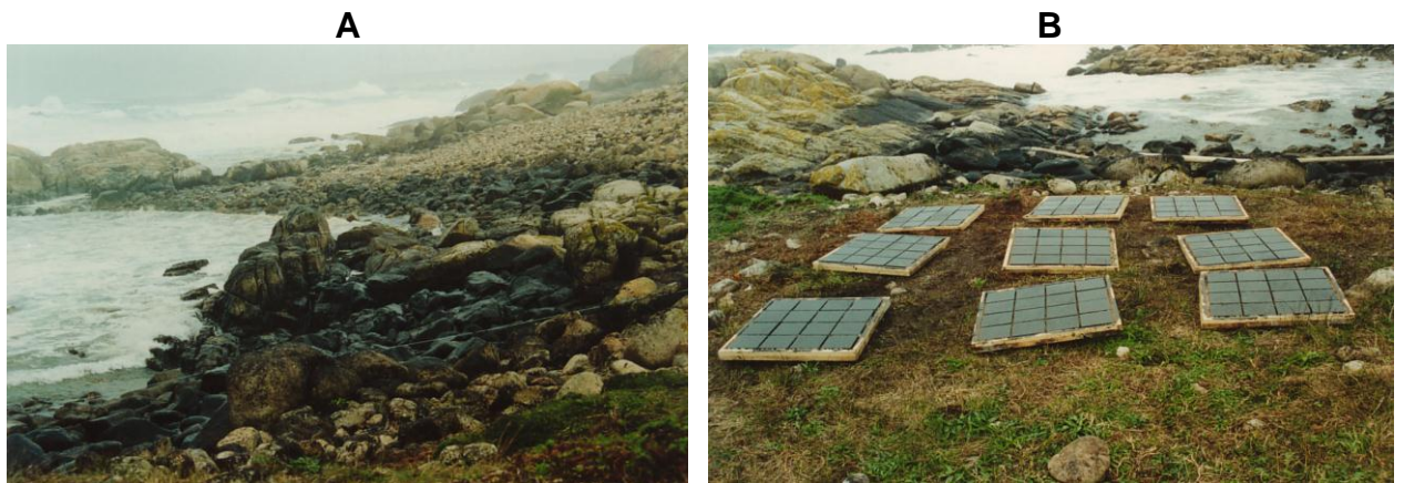
Figure 1. A: Detail of the treated area (high tide). B: 9 of the 60 panels of granitic tiles impregnated with fuel from Prestige that were used for quantifications.
